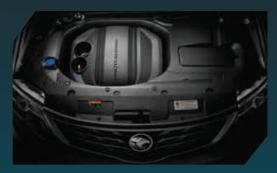
1.5L TGDi, 3 Cylinders In-Line, 12 Valve DOHC, Turbocharged Petrol Engine
