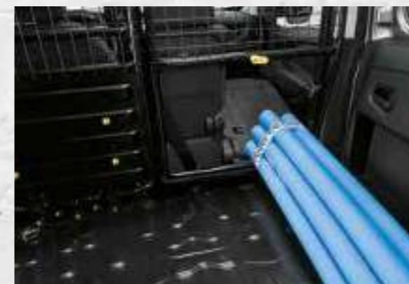
Multi functional partition for 3 seats configuration, removable on passenger side to accommodate long objects
