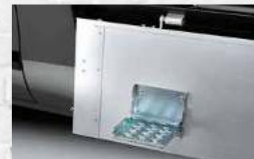
INTERNAL STEPS FOLDING INTO SIDEBOARDS
