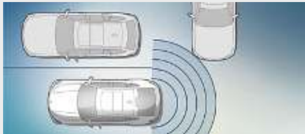
□ The Crossing traffic warning rear* warns you of crossing traffic when pulling out of perpendicular parking spaces.
