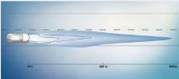
□ BMW Laserlight in a unique X design reaches a maximum illumination range of up to 500 m in laser high-beam mode.
