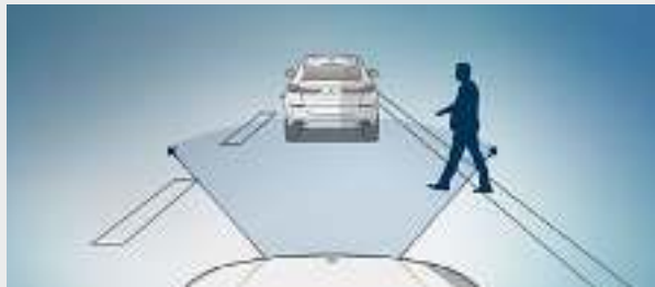
□ Active Guard* includes the front collision warning with braking function and Lane Departure Warning.
