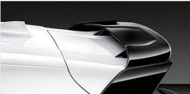
○ Moving design. The M Performance roof spoiler is made of PUR in Black high-gloss, an elegantly athletic accent for the rear of the vehicle. At the same time, it contributes to optimised aerodynamics. The spoiler is perfectly tailored to the vehicle design and can be painted in the body colour.
